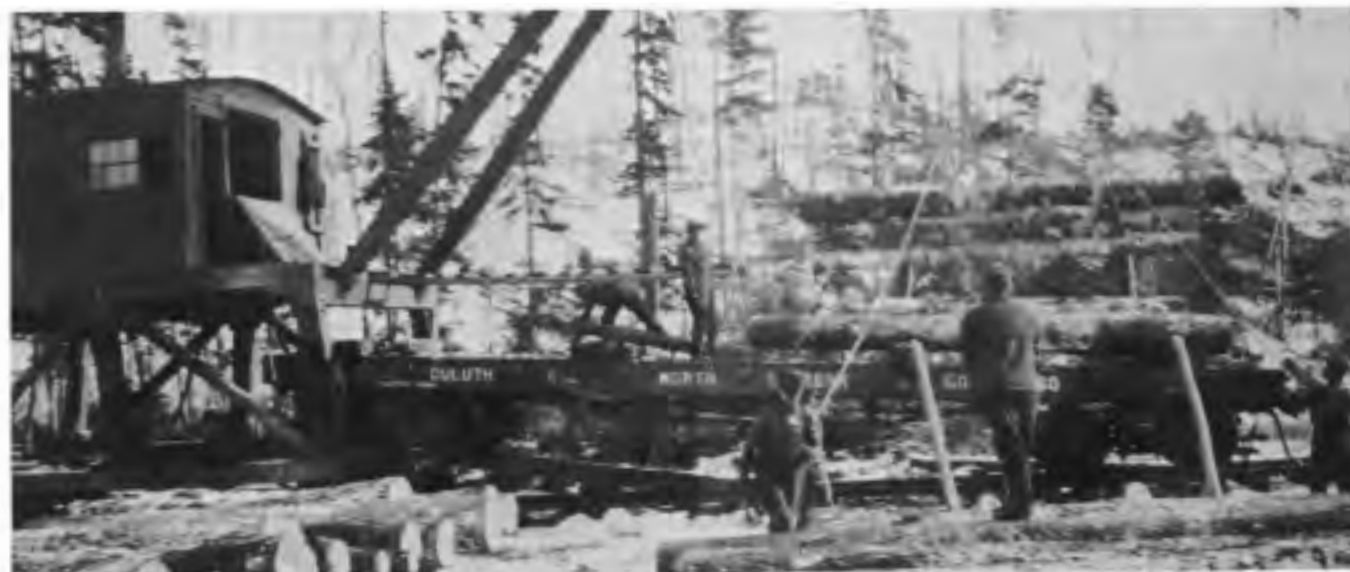
Steam jammer pulled flatcars through as it loaded them. A good crew loaded 18 cars a day.
