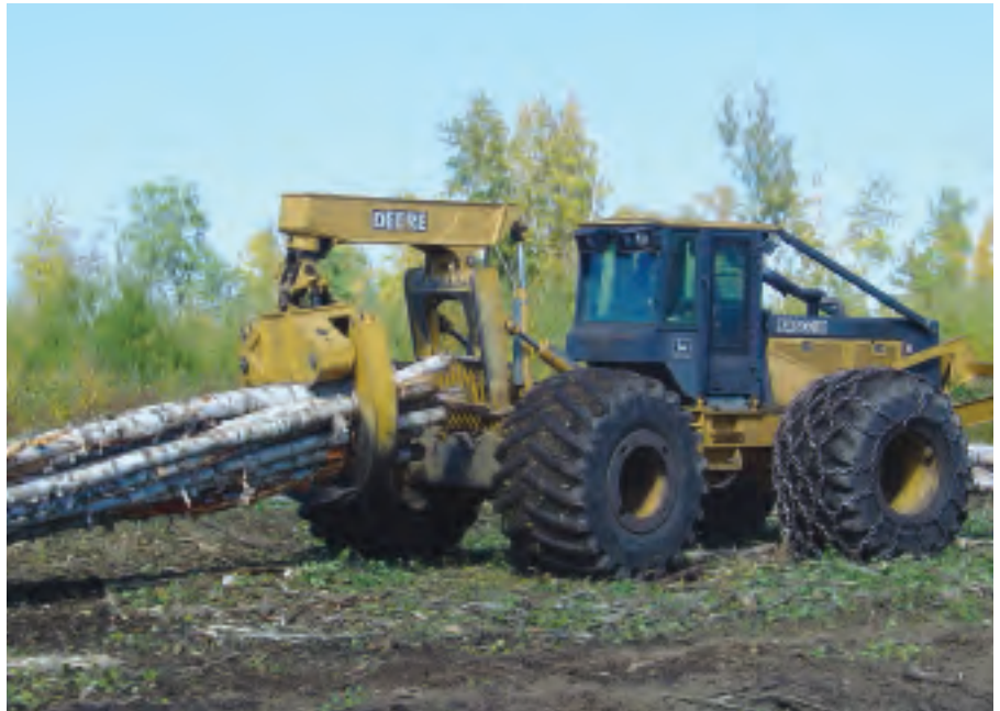
Eric Peterson skids with one of the company's two John Deere 748 G3 skidders.
