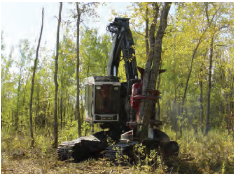
Jon Peterson operates Peterson Logging's Timbco 425D feller buncher in an aspen stand north of Williams.
