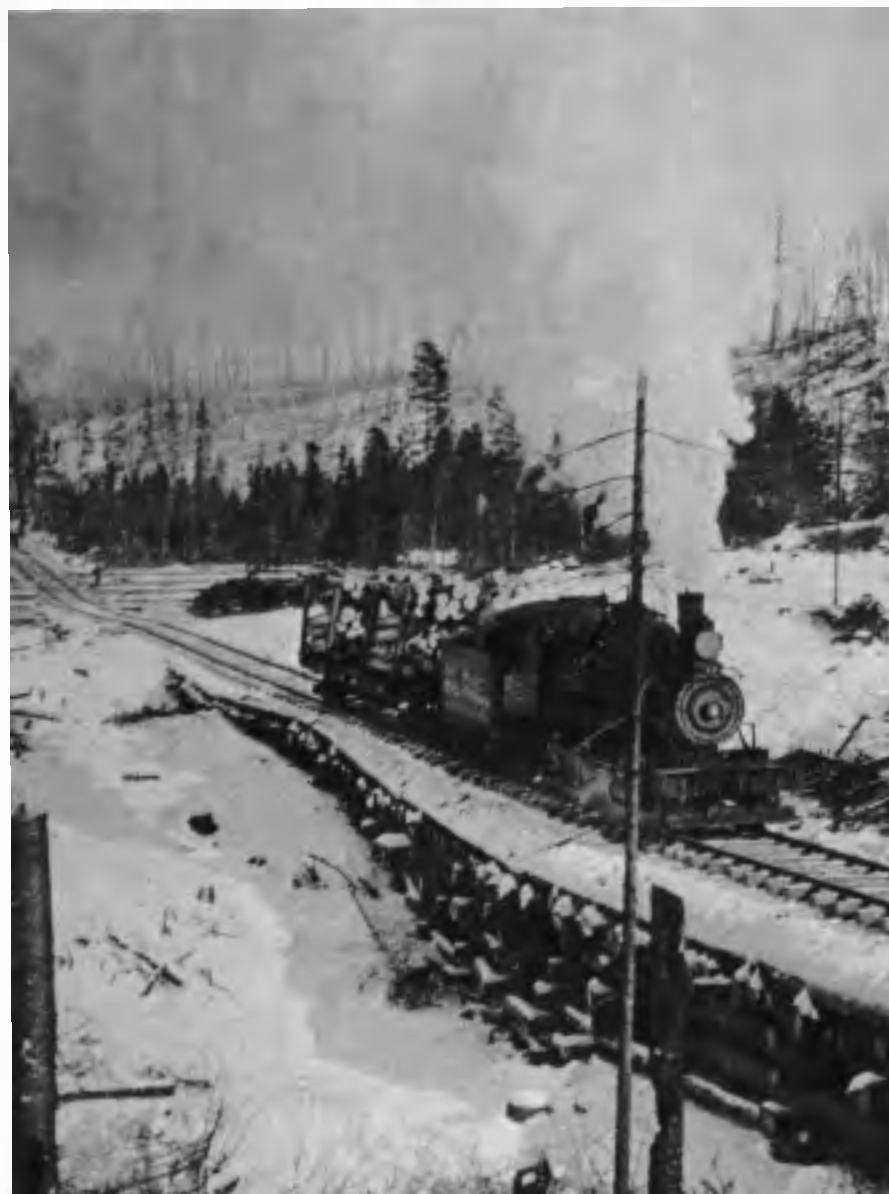
Blasting up a steep grade, a Duluth and Northeastern engine moves one flat of logs at a time, as steam jammer at the end of the spur taster another car. Uninsulated track and fill work in the deep cut were typical on these temporary spurs.
